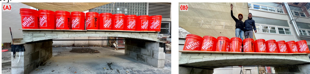
Figure 12: (a) Prototype under uniform load of 2 \text{ kN/m}^2 ; (b) uniform load and human point load totaling 1.25 \text{ kN}
