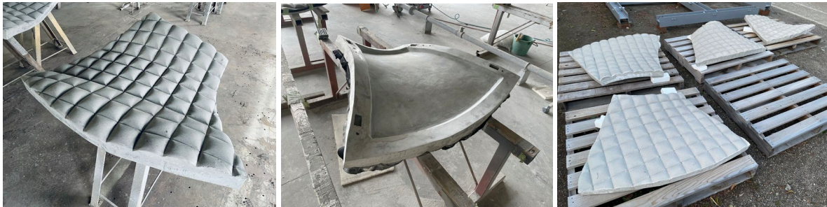
Figure 9: Appearance of the demolded GFRC panels
